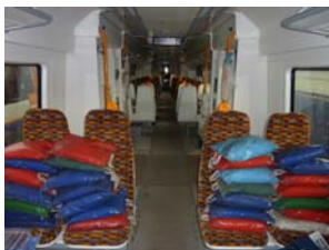
Looking to the rear of 59311 & into 59411. Note the 'sand-bags' to simulate a loaded train and test equipment.
